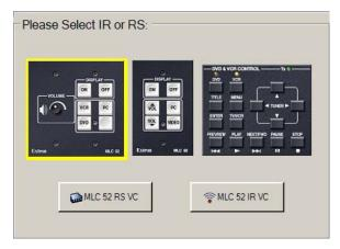
MLC driver type selection buttons on the device selection screen
